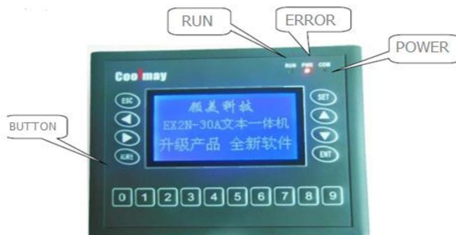
30A has 18 function buttons and can be defined with specific function.
